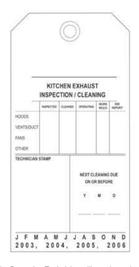
The Tag has the months and year at the bottom. The Fire Protection Technician will punch out the month in which the test/inspection is done or date the Tag under the Stamp.
