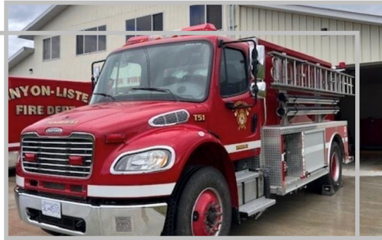
Tender 51 - Canyon Lister - 2011 Freightliner (Rosenbauer) with 650 gpm pump and 1,600 gallon tank.
