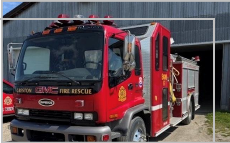
Engine 61 - West Creston - 2001 Superior Pumper- 1,050 pump with 800 gallon tank.
