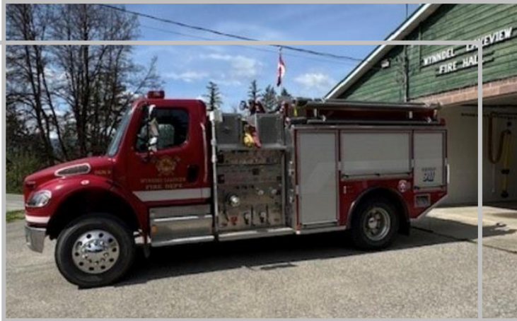
Engine 41 - Wynndel-Lakeview - 2000 International Pumper- 1050 gpm with 500 gallon tank.
