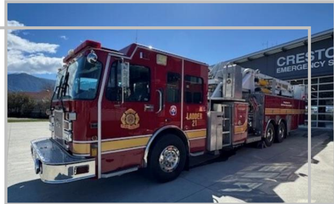
Ladder 21 - Creston - 2001 Quint with 1500 gpm pump and 500 gallon tank
