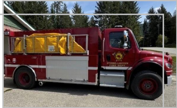
Tender 41 - Wynndel Lakeview - 2020 Freightline with 650 gpm pump and 1,600 gallon tank.
