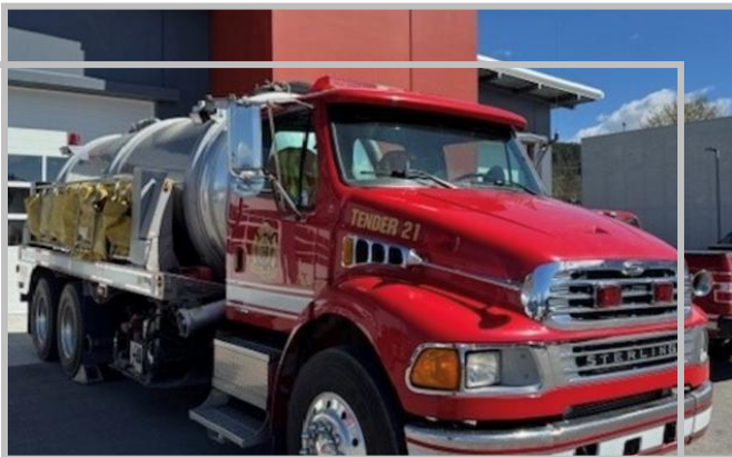
Tender 21- Creston - 2003 Sterling Water Tender with 3,000 gallon tank.
