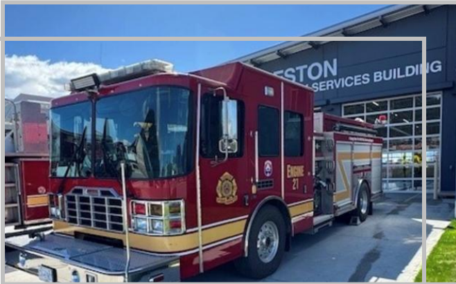
Engine 21 - Creston - 2010 Ferrara 1500 gpm pumper with 1,000 gallon tank
