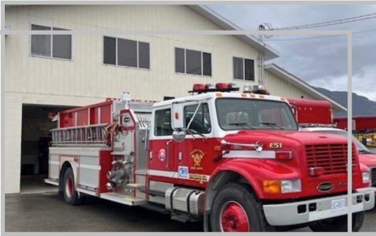
Engine 51 - Canyon Lister - 2000 International Pumper with 1050 gpm and 800 gallon tank.
